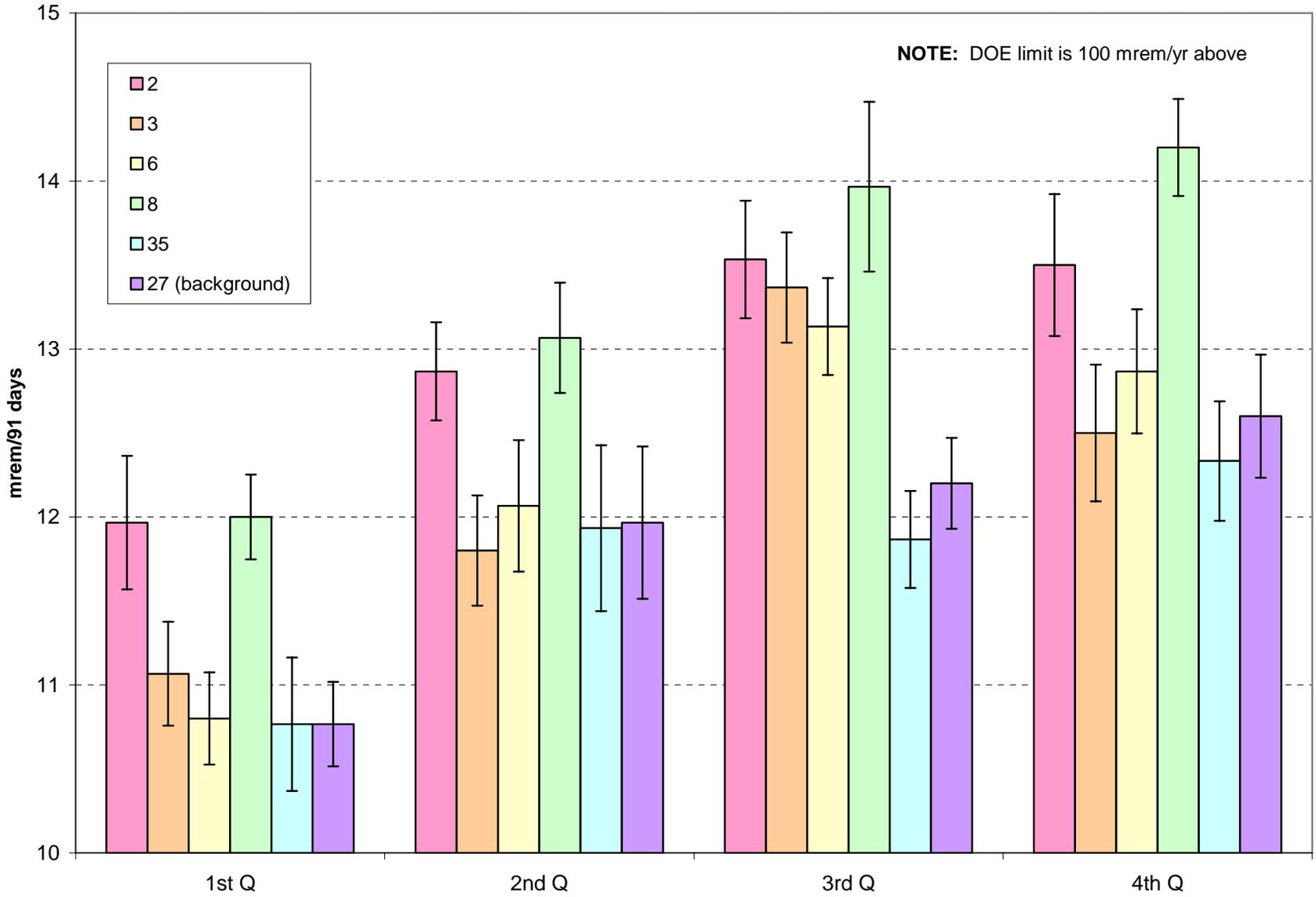
Figure 5-7. Quarterly Results and Measurement Error Recorded by TLD Monitoring Location
