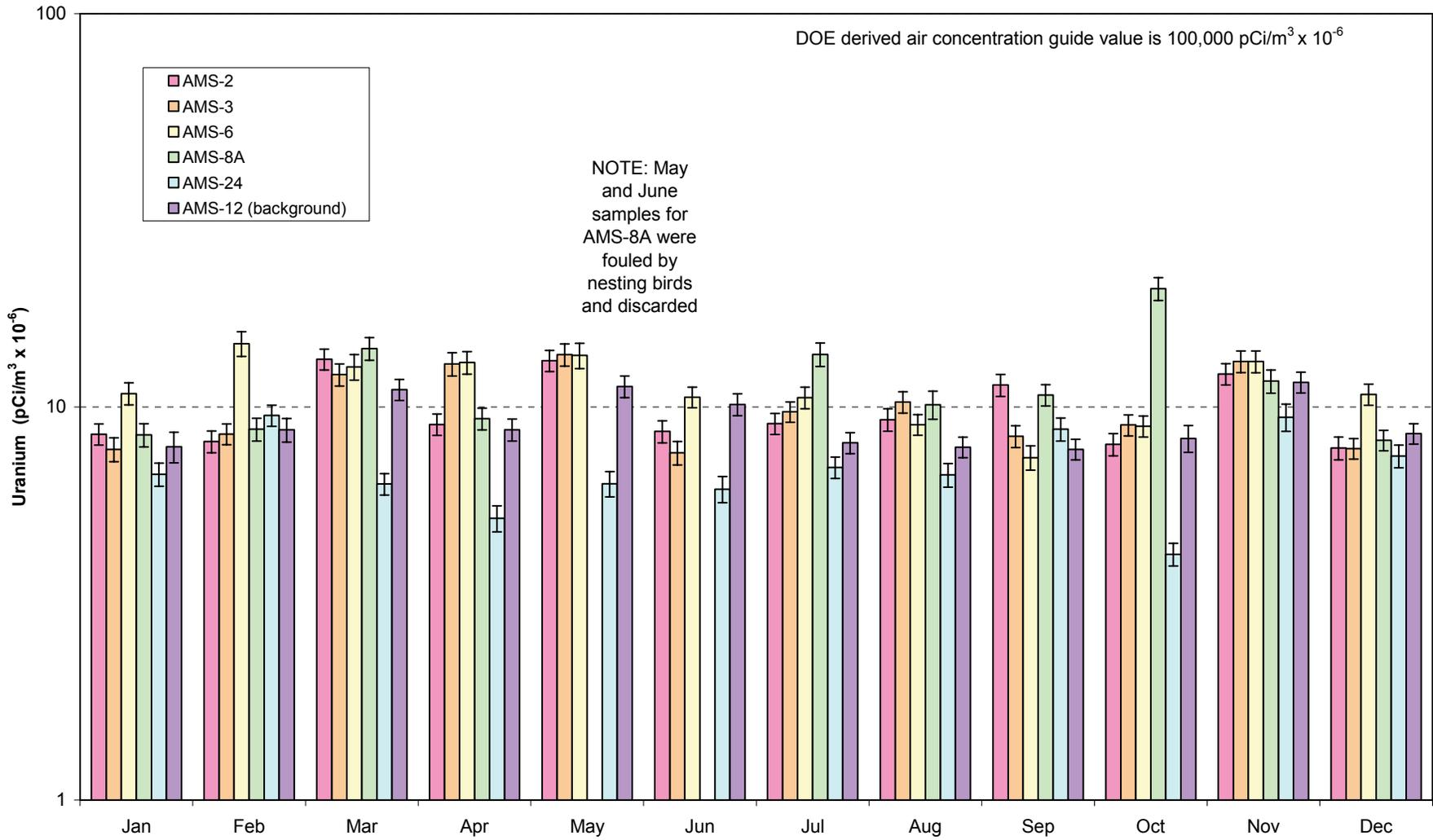
Figure 5-2. Monthly Results and Measurement Error for Uranium in Collected Air Particulate
