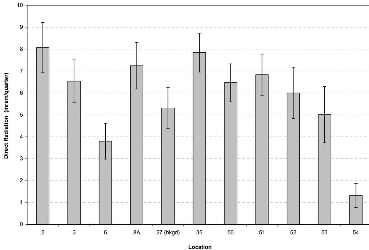
Figure C.1–2. 2012 Mean and 95 Percent Confidence Interval for Quarterly Dosimeter Measurements
